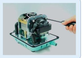
Remove 2 U-lock nuts from one side holding the diaphragm mounting block to the rod.
