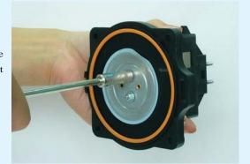
Insert the actuating rod into the machine body. Be sure to fit the positioning boss on the diaphragm base into the concave part of the frame stay.
